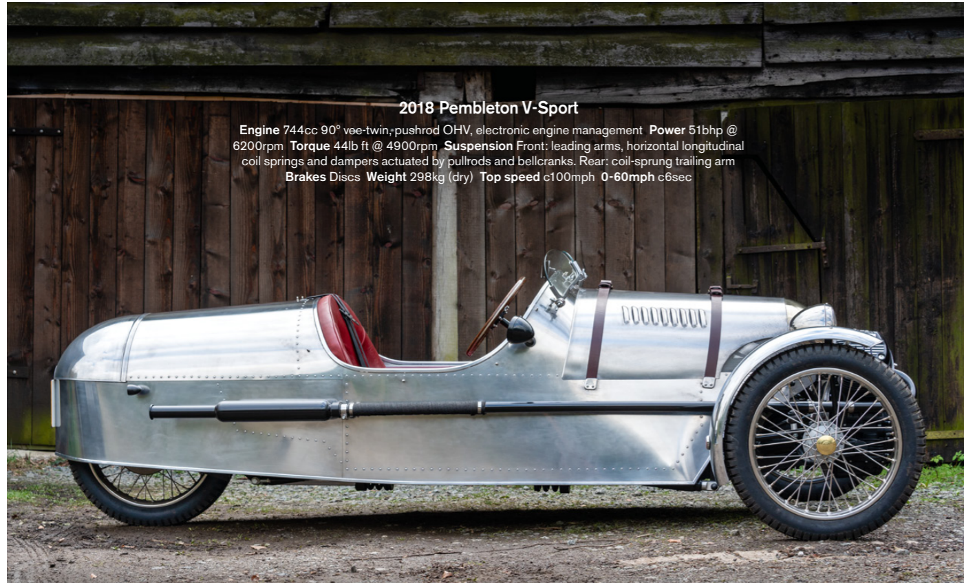
Clockwise from above V-Sport is beautifully made with laser-cut panels; name came from a caravan; roomy cockpit is ultra-simple; Guy Gregory (on right) has re-imagined original design of father Phil (on left).
